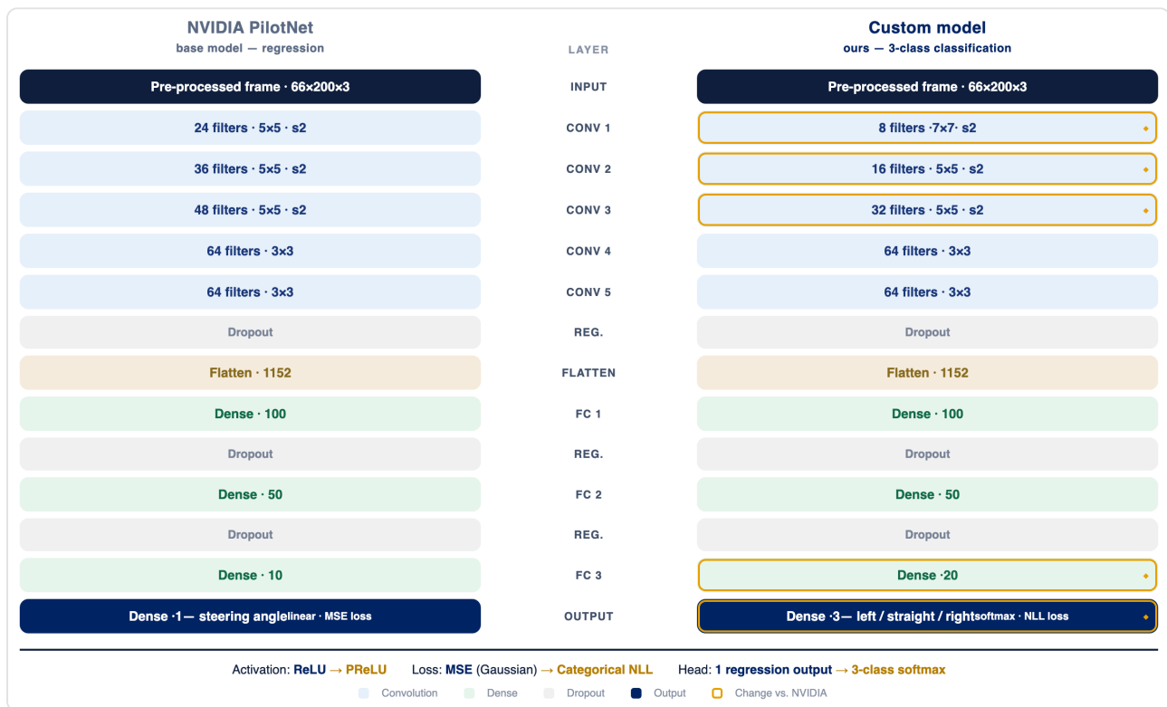
Fig. 1. NVIDIA PilotNet (base) vs. the custom model. Amber-outlined blocks mark the changes: a wider first kernel, a lighter convolutional stack, a wider penultimate dense layer, and a 3-class classification head with a categorical NLL loss; ReLU is replaced by PReLU throughout.
